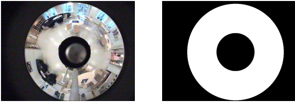
Fig. 1. left: Example panoramic image. right: Pre-defined mask to cut out the used pixel-ring.
