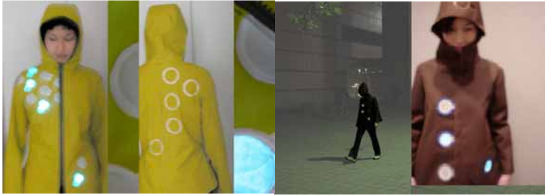
Figure 8: Mintymonkey's Puddlejumper is a luminescent raincoat that glows in the rain. Hand-silkscreened electroluminescent lamps on the front of the jacket are wired to interior electronics and conductive water sensors on the back and left sleeve. When water hits one of the sensors, the corresponding lamp lights up, creating a flickering pattern of illumination.
