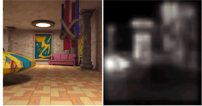
Figure 3 The image on the left shows a screen capture of an animated sequence. The image on the right shows the corresponding activation map. The brighter areas on the map show regions of higher visual importance [Yee 2001].
