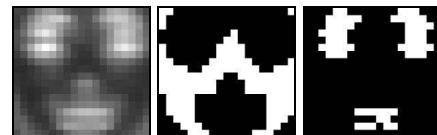
Figure 1 Example ensemble wavelet decompositions are shown for (left) horizontal coefficient image, (middle) horizontal low threshold and (right) horizontal high threshold coefficients.
