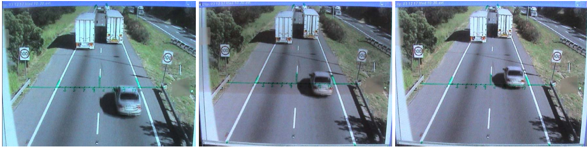
Figure 2: Screen shot as the a) front of the vehicle crosses the reference line b) widest part of the vehicle crosses c) rear of the vehicle crosses
