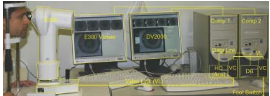
Figure 1. Equipment set-up for high-speed (50 Hz) videokeratology. VC: video card, VL: video link, DB: data base, HD: auxiliary hard drive.
