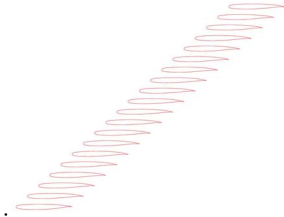
Figure 7. The Ensemble of Pareto Aerofoils.
