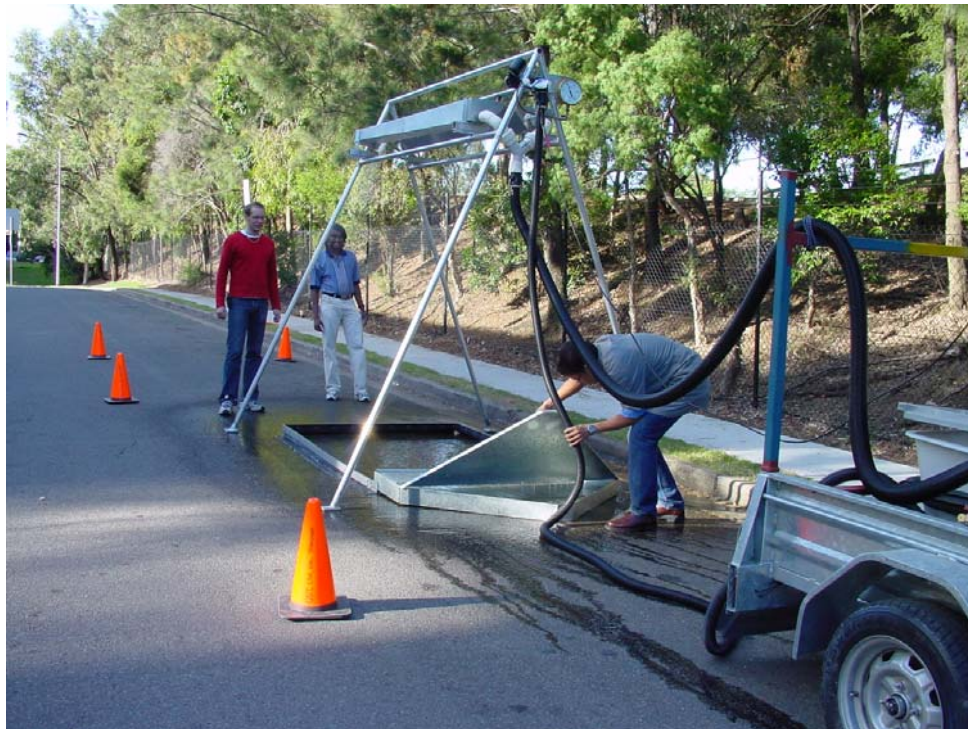
Figure 1 – The developed rainfall simulator
