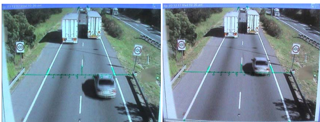
Figure 5: Screen capture as the a) front of the vehicle crosses the reference line b) rear of the vehicle crosses the reference line
