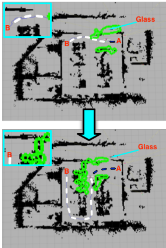
Fig. 5. A to B using the proposed approach. Each panel representing the robots navigation state at stages during the same run. Black represents occupied space of the hypothesis. Green represents the observed obstacle boundaries with a safety margin (inflated obstacles). Enchantments added for the reader include: Letters 'A' and 'B' for starting and goal locations. Blue dash's for plan completed and White plan under current action.
