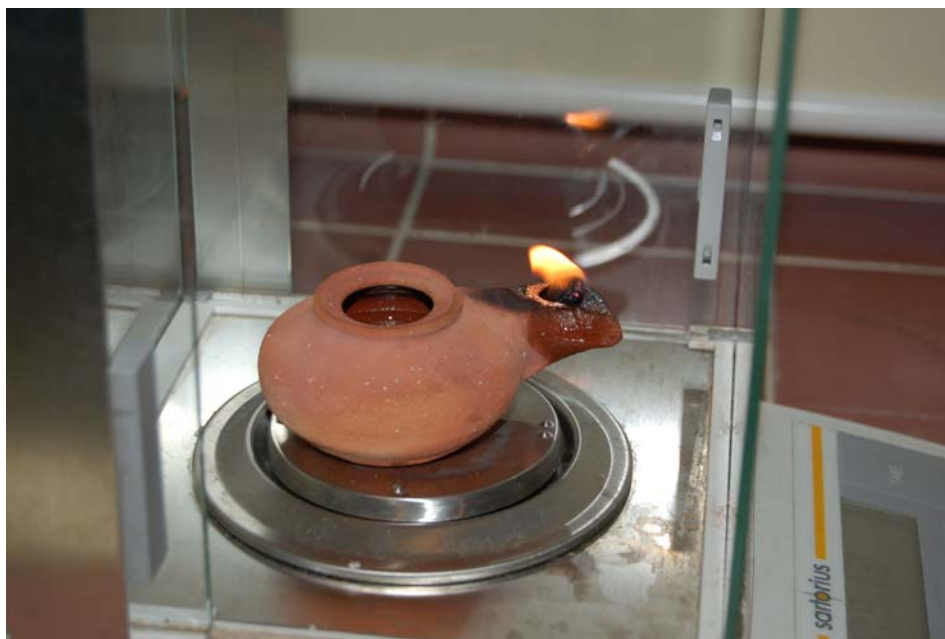
Figure 2. Oil lamp on an electronic balance, to measure the fuel consumption rate.
