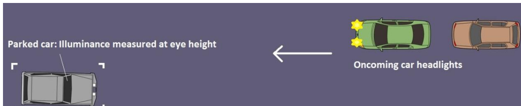
Figure 5-2: Position of experimental vehicle and oncoming traffic for measuring at-eye illuminance of oncoming headlights at night
