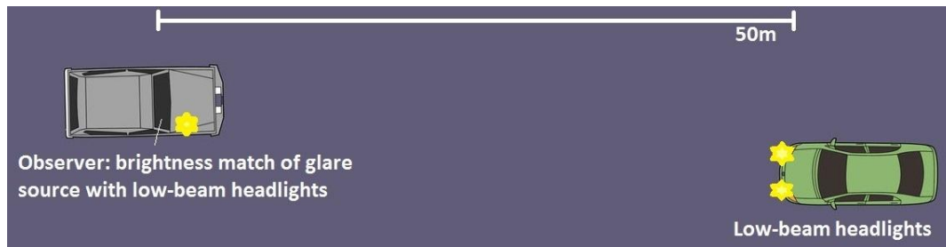
Figure 5-3: Position of glare source and real car headlights for subjective brightness matching
