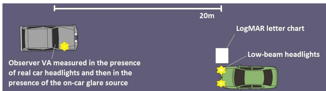
Figure 5-4: Position of the observer, on-car glare source, low-beam headlights and VA chart
