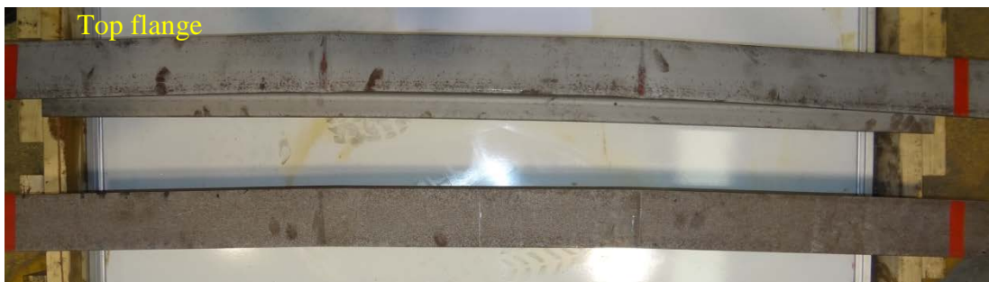
Figure 4.32: Failure mode of B300-A specimens
