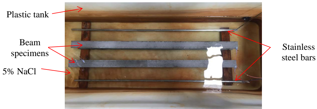
Figure 3.18: Laboratory accelerated corrosion cell setup
