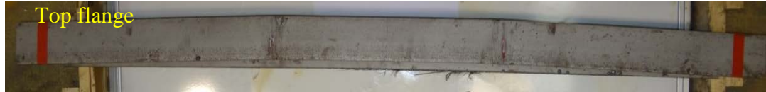
Figure 4.33: Failure mode of B300-B specimens
