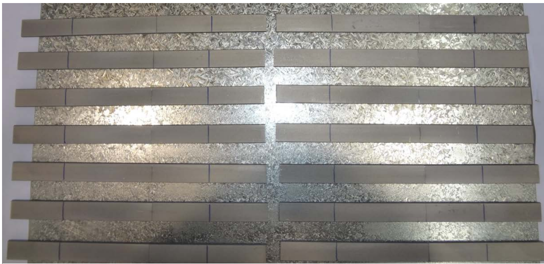
Figure A1: Sandblasted specimens cleaned with acetone
