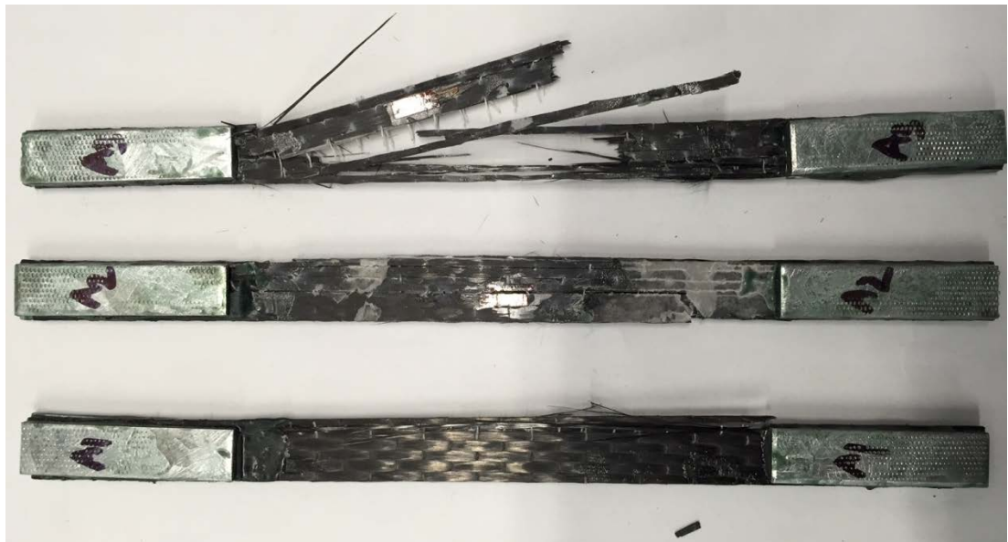
Figure C1: Failure modes of CFRP coupons
