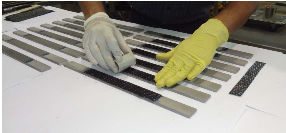
Figure A4: CFRP installation
