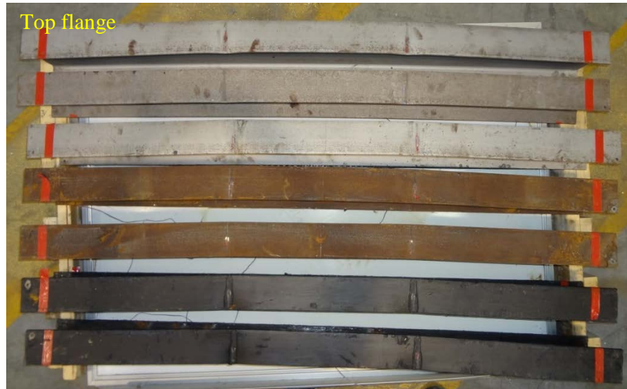
Figure 4.36: Comparison of failure modes of beam specimens
