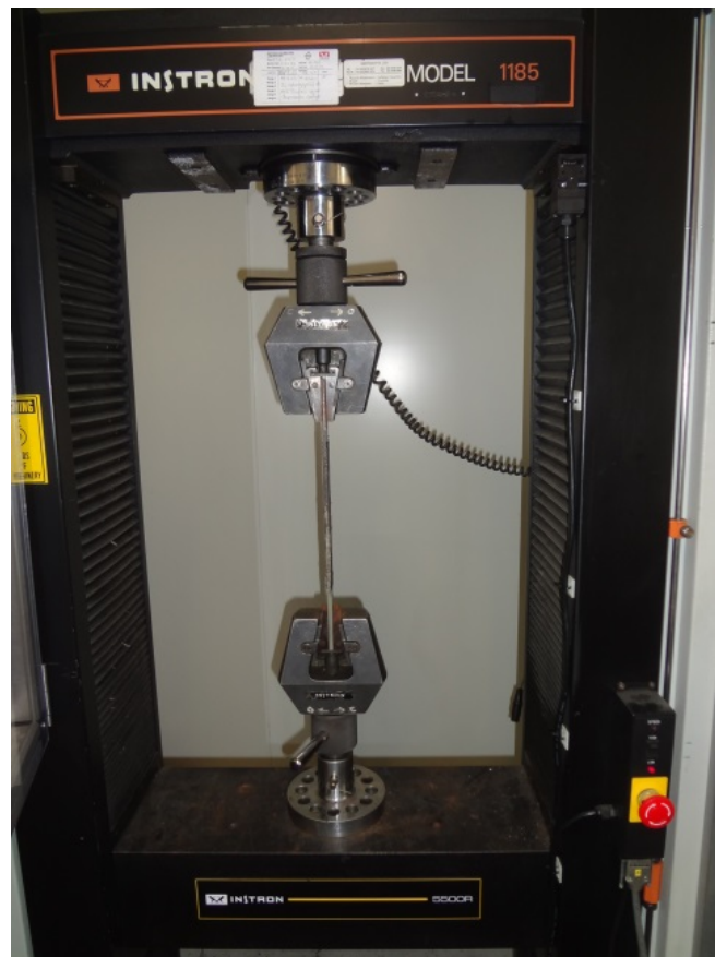
Figure 3.6: Tensile loading set-up
