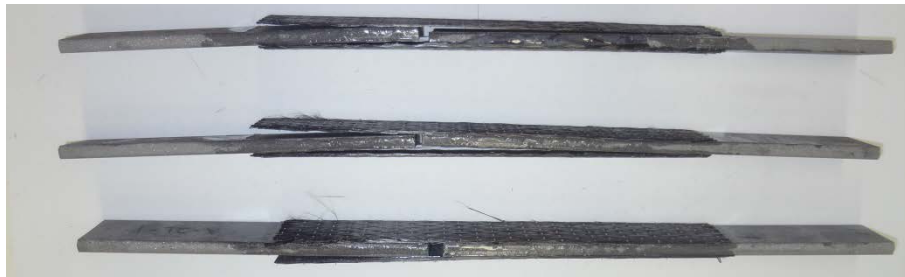
Figure 4.1: Steel-adhesive interface debonding of double-strap joints
