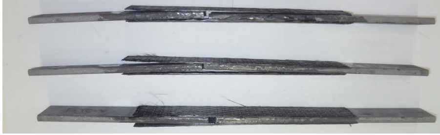
(a) Debonding failure - experimental
