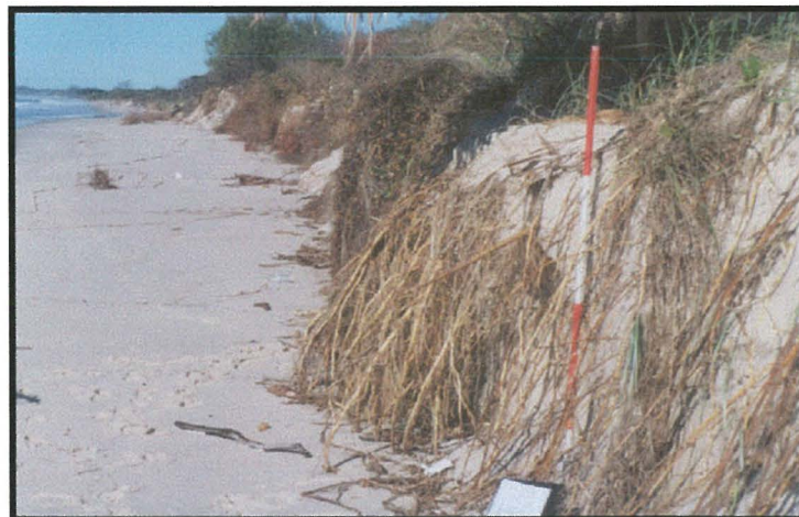
Figure 29. Undercutting and slumping of the erosion scarp occurring approximately one month after the flattening of the beach profile by the April storm due to the lack of a built up beach profile.
