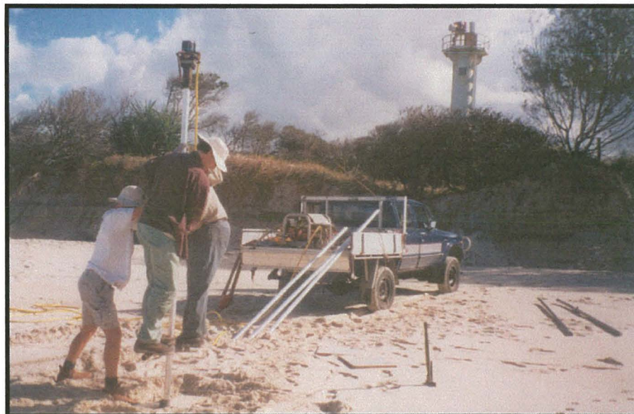
Figure 21. Vibrocoring at section B-B'. Equipment mounted on 4WD for access.
