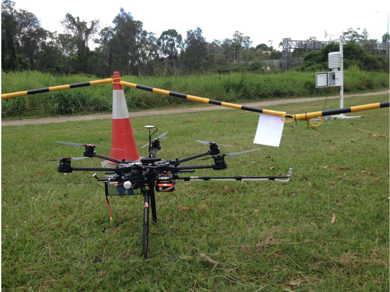
480 Figure S1: The UAV system. the DJI S800 UAV with the DISCmini mounted onboard.
