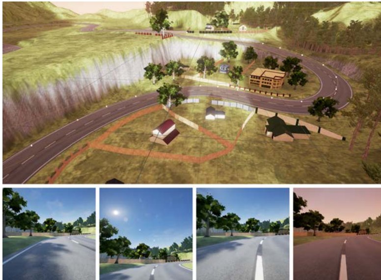
Fig. 1. The custom street scene used to capture the image datasets that were used for testing the place recognition algorithms. The line of white dots shows the baseline path followed by the camera when generating the datasets to test Sum of Absolute Differences and SeqSLAM place recognition performance. The SLAM experiments followed a slightly different path in order to ensure a complete loop of the environment.
