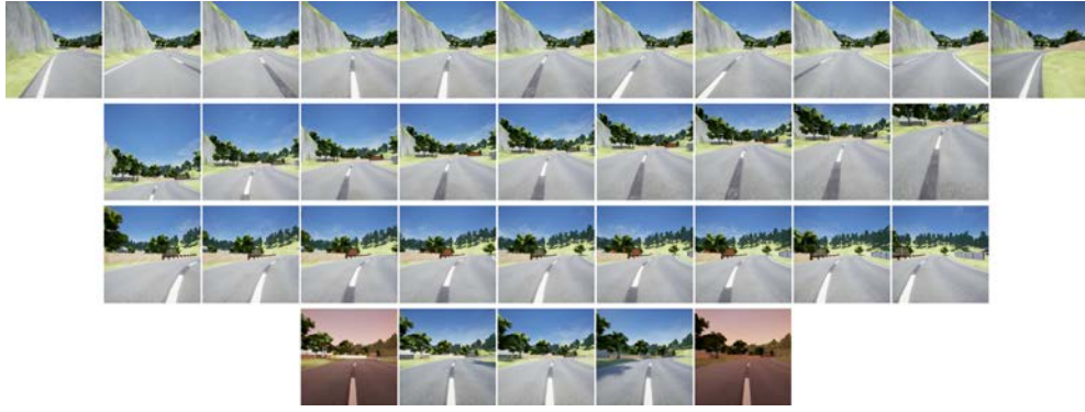
Fig. 2. A Sample of the variation found in the datasets used for testing. The first row shows lateral offset, from left to right, images are offset are left 3.5m, 2m, 1m, 0.4m, 0.2m, Then the baseline, then offset right 0.2m, 0.4m, 1m, 2m, and 3.5m. The second row shows vertical orientation change, left to right, images are angled are up 30^\circ , 15^\circ , 10^\circ , 5^\circ , Then the baseline, then angled down 5^\circ , 10^\circ , 15^\circ , and 30^\circ . The third row shows horizontal orientation change, from left to right, images are angled are left 30^\circ , 15^\circ , 10^\circ , 5^\circ , Then the baseline, then angled right 5^\circ , 10^\circ , 15^\circ , and 30^\circ . Finally, the lowest row shows samples of time of day variation, from left to right, images are taken at dawn, in the morning, at noon, in the afternoon, and at sunset.
