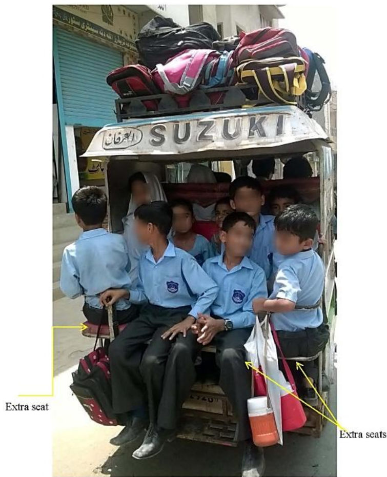
Figure 6.3: Modifications in MR design to carry extra passengers and weight (Source: Author, 2015)
