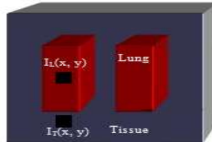
Figure 4-4: The model lung phantom showing the region of interest (black square) used to calculate the contrast before and after calibration in the simulated images.
