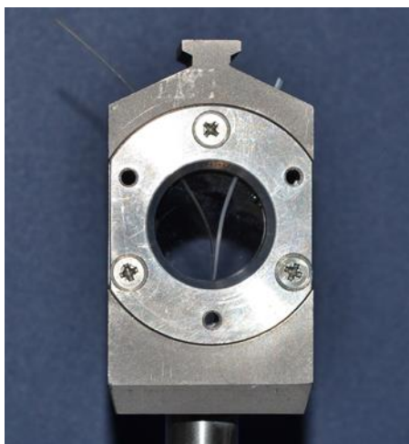
Figure 3-2. The 2 mm QUOKKA cell placed on the DINGO platform. Two strips of Nafion inserted into the cell forming a "V" shape.
