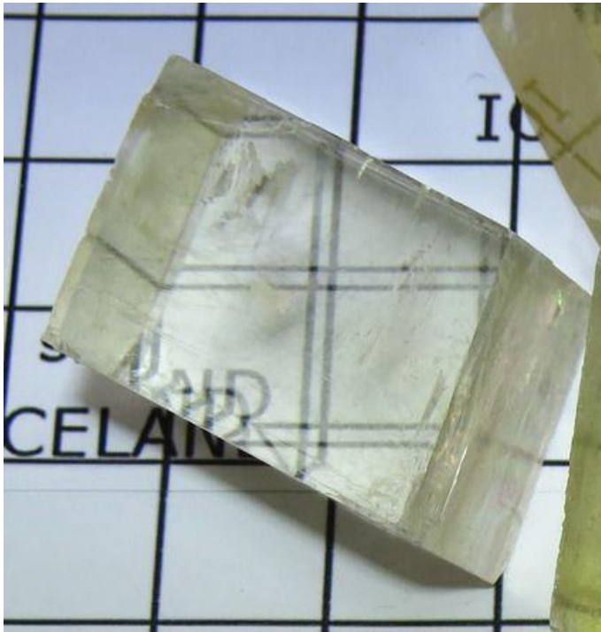
Figure 3-13. Calcite crystal displaying distinctive double refraction of underlying image. (Summers 2015).
