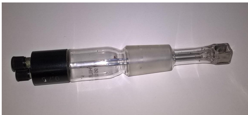
Figure 3-29. Philips PW9512/01 cell with platinised platinum black electrodes.
