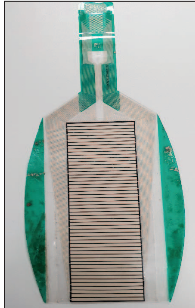
Figure 4-5 Image of pressure sensor used in this experimental design
