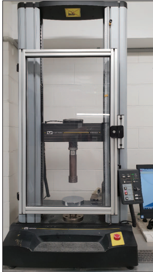
Figure 4-3 Image of 50 kN Instron Universal Testing Machine used for both CBR and tensile tests
