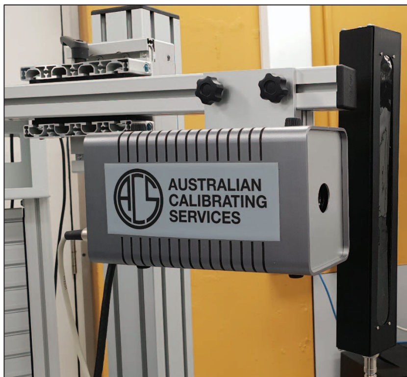
Figure 4-15 Image of Video Non-Contact Extensometer (VNCX) used in this research for measuring strain in tensile tests
