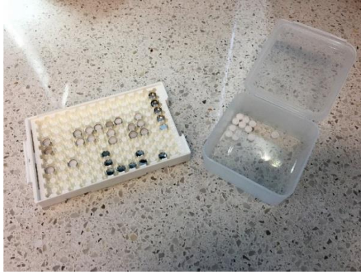
Figure 6: Platinum Crucibles Lined with Alumina Liners and Pin Holed Lids
