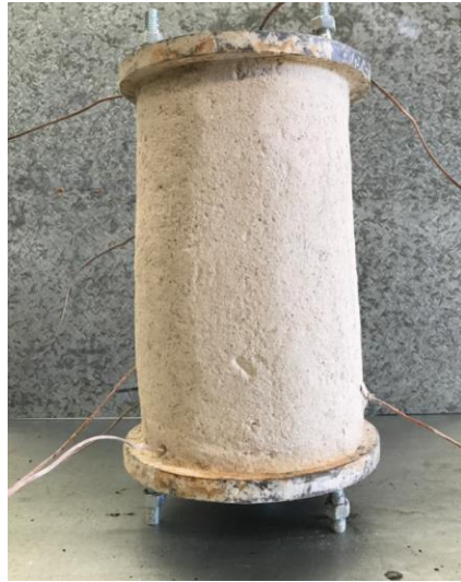
Fig. 5. CFRP strengthened and insulated column
