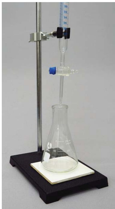
Figure 6.4 Quantification of active sites: titration setup
