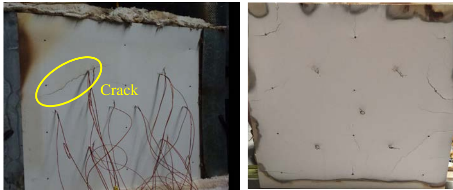
(a) Cracking and discolouration of ambient side board
