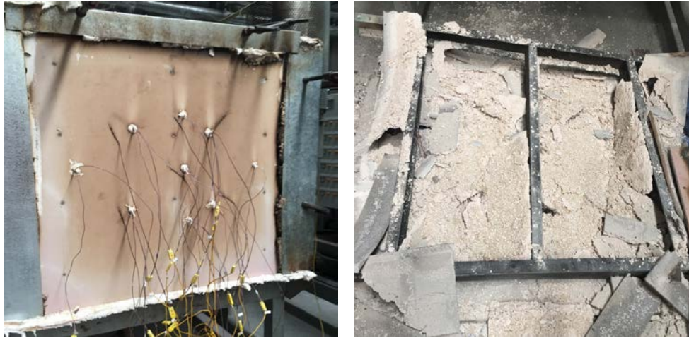
(a) Discolouration of ambient side plasterboard (b) Plasterboard and stud after the test
