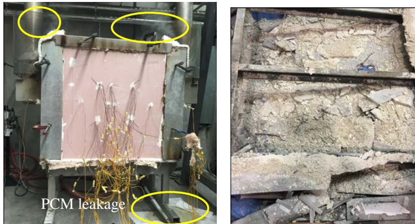
(a) Smoke and melted PCM leakage (b) Discolouration and fall-off on the fire side after the test
