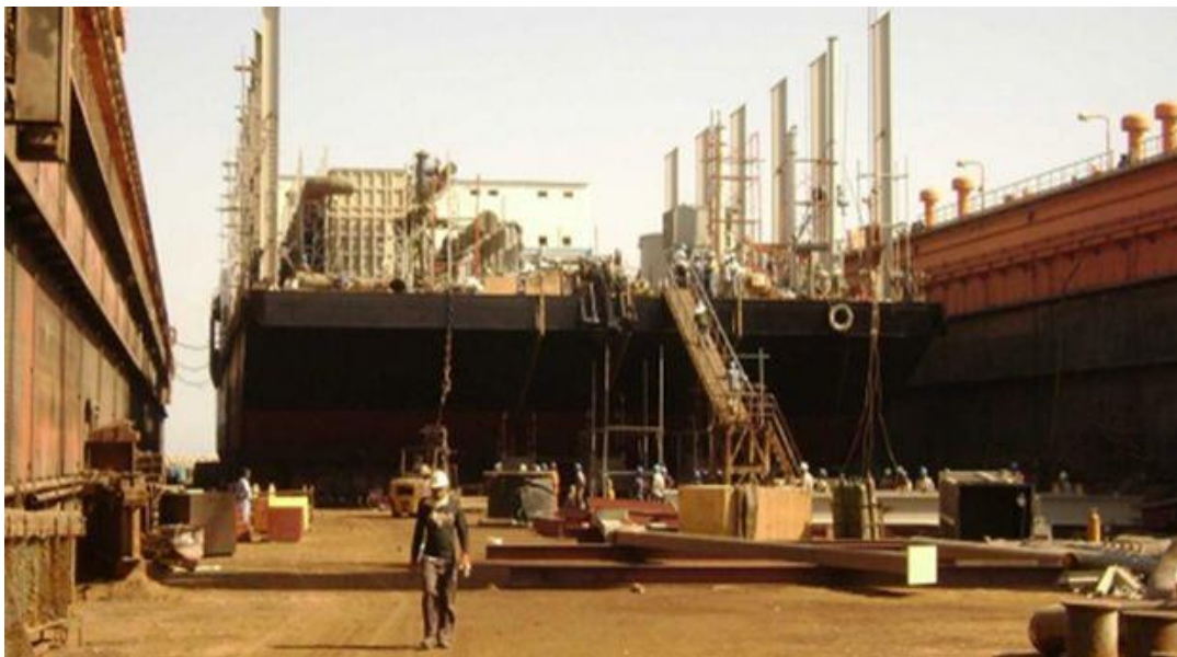
Fig. 8 Floating desalination plant at Jeddah
