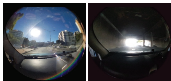
Figure 1: shows the black hole effect and the white hole effect found when approaching and exiting the tunnel in images taken with a fisheye lens.
