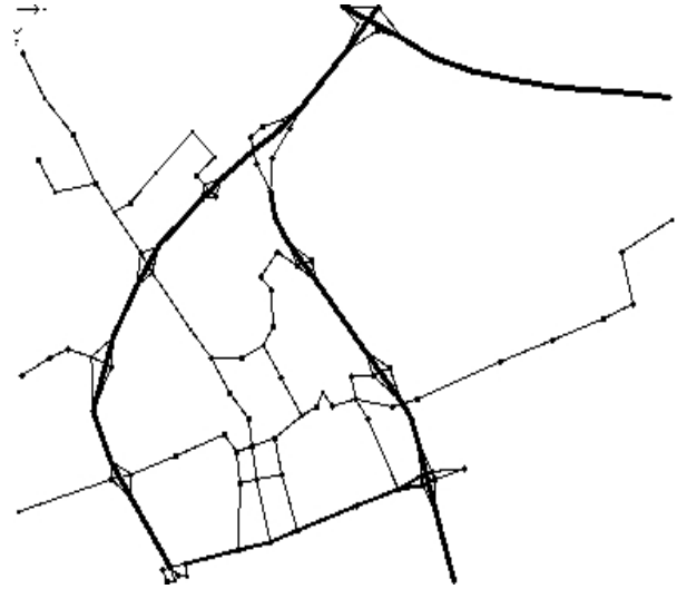
Fig. 3. Delft network with two highways around the city and an urban connection in the south, as well as the major urban roads of Delft.
