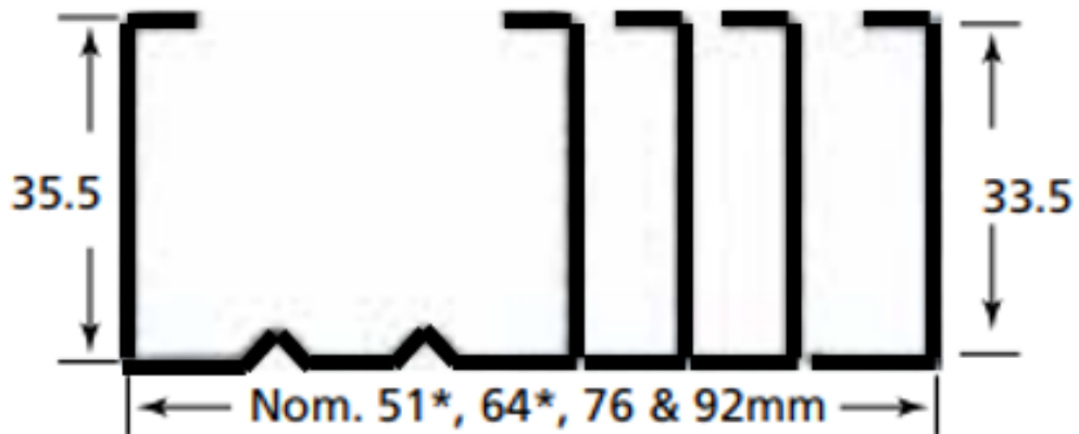
Fig. 3. Basic LSF wall stud geometries [15]
