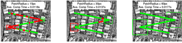
Fig. 8. A visual indication of the performance of the calibration procedure on a traversal across the Nearmap 8b dataset. As can be seen the optimal patch radius selected by the calibration procedure, 30 pixels, results in almost perfect recall with a much lower computation time per iteration compared to that of the traverse using a 60px patch radius. Each green and red dot indicates the center of query patch and whether it successfully or unsuccessfully localized itself within the reference map respectively.
