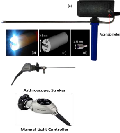
Fig.8. The stereo endoscope prototype (a) together with the close-up view at the tip (b) and the 3D design (c) and the muC103A camera (d). The potentiometer shown by the red arrow is used to adjust the LED intensity. The endoscope circuits and extra wiring are contained inside the black box and connected to the computer using two USB cables.
