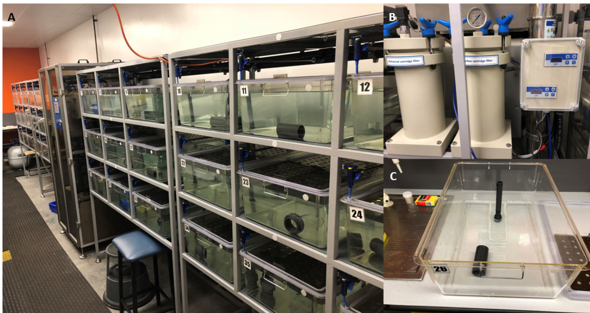
Figure 20: A - Techniplast Xenoplus Multi-linking Water Treatment System. B - Internal Mechanical filter, Carbon Filter, pH and Conductivity Probes and UV Steriliser. C - Example of a 27L tank used in the system with the inbuilt overflow drain.
