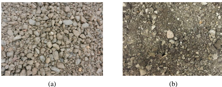
Figure 1. (a) Recycled concrete aggregates-RCA (Scale 1:5) (b) Reclaimed asphalt pavement-RAP (Scale 1:3.2)
