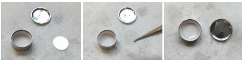
(b) 0.25 mm (20.6 mg and 20.9 mg) sapphire disc placed in the crucible
