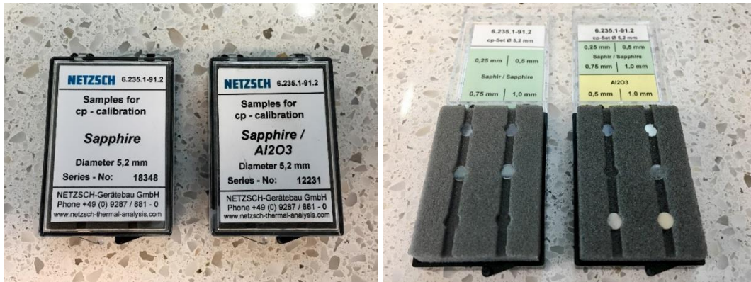
(a) Different sizes of sapphire discs supplied by NETZSCH
