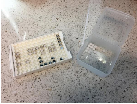
Figure 3: Platinum Crucibles Lined with Alumina Liners and Pin Holed Lids
