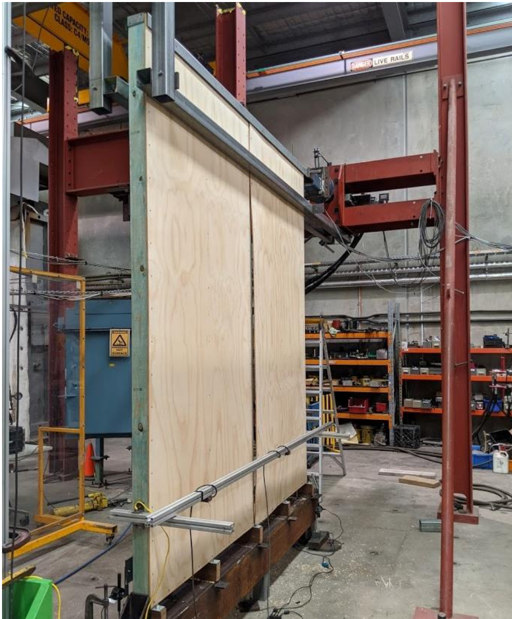
Figure 21: Test Panel C4.3 After Failure.
