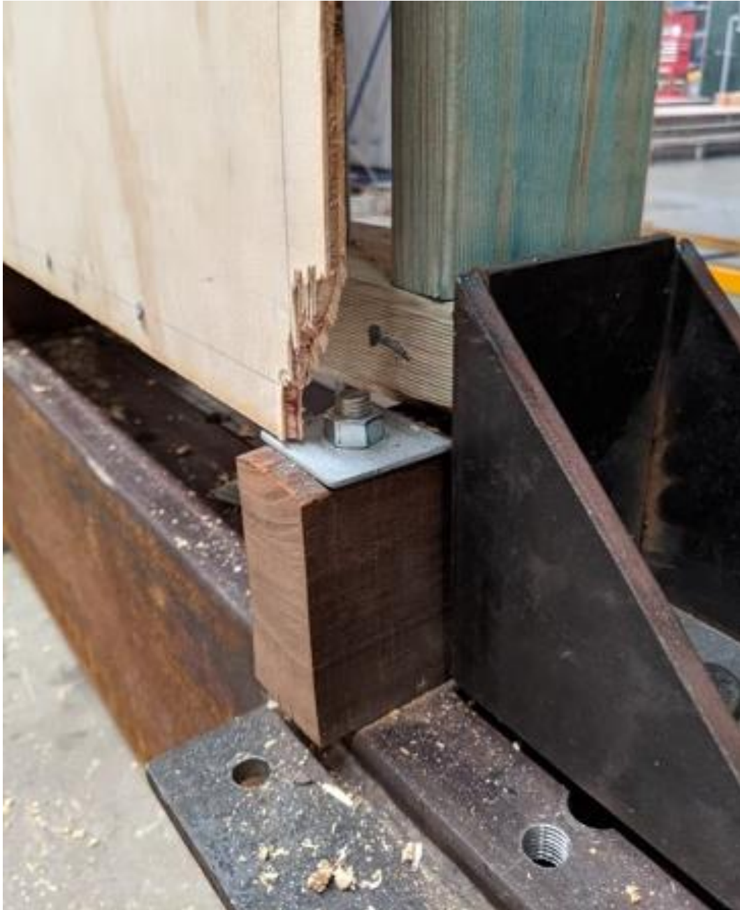
Figure 20: Test Panel C4.2 After Failure.
