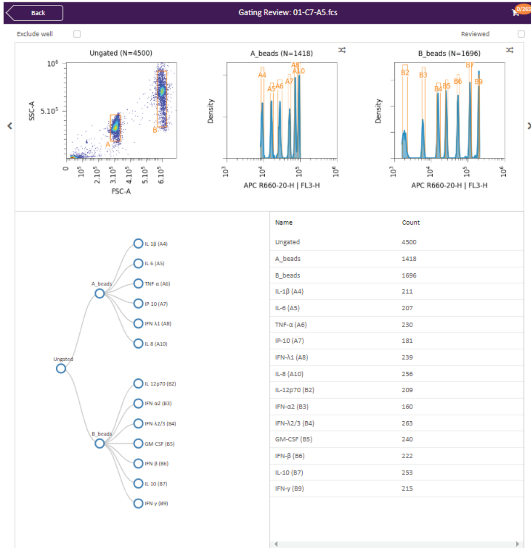
Figure 2.1.3 Gating of two populations of Legendplex beads (A and B) of the top standard (C7) with 4500 events recorded. Panel used was the Legendplex Human Anti-Virus Response Panel, tested with the Cytoflex S flow cytometer and analyzed using the Legendplex Qognit software.
