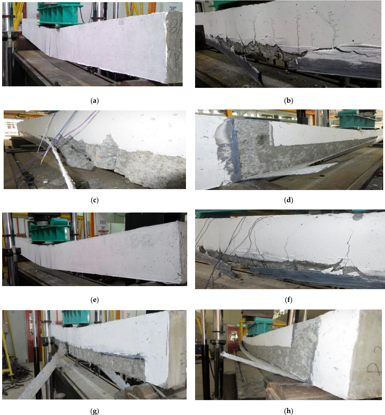
Figure 8. Failure modes of the beams; (a) CB-A; (b) SE-A; (c) SE-2A; (d) SE-3A; (e) CB-B; (f) SE-B; (g) SE-2B; (h) SE-3B.
