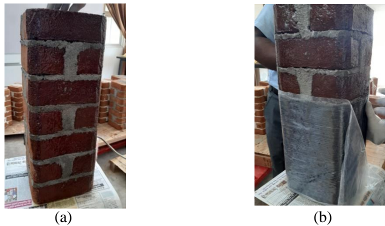
170 Fig 2. Application of CFRP sheets to the masonry columns (a) Epoxy coating and (b) wrapping of CFRP sheets.
