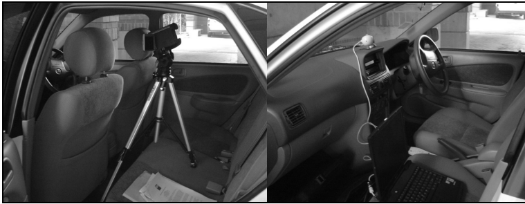
Figure 7-4. Mini DV camera and tripod set-up (left) and Webcam and Laptop set-up (right) (Gomez et al. 2004a).
