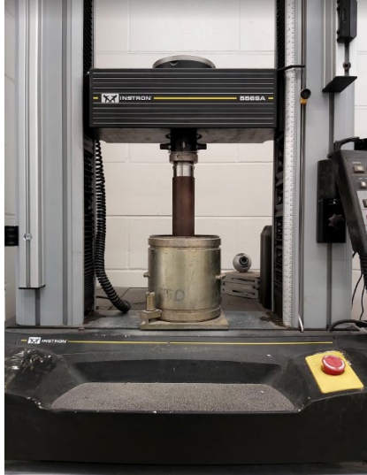
Figure 2: Performing standard CBR test using Instron machine.
