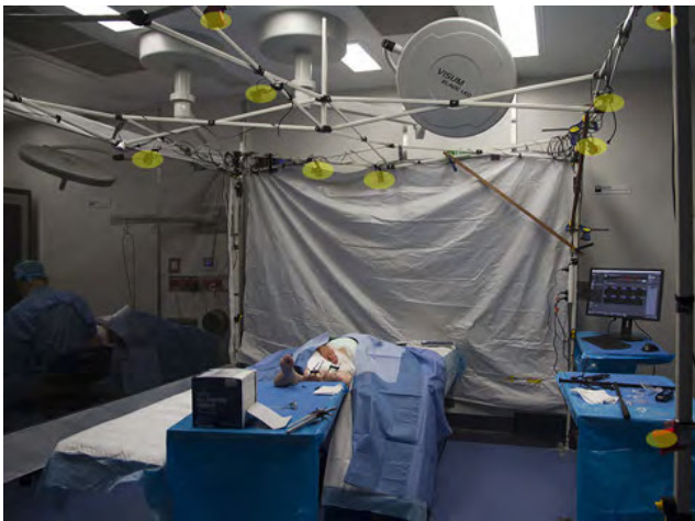
FIGURE 3. Optical Tracking volume setup for Cadaver experiments. Ten cameras (the visible camera is highlighted in yellow) are fitted to a frame that was setup around the cadaver. Cameras were installed at specific points to ensure visibility of the arthroscope from at least three cameras during surgery. Blanking screens are installed to limit reflections.
