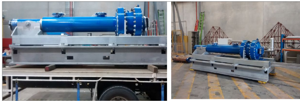
192 193 Figure 6: Barrel with attached pressure vessel arriving from manufacture ready 194 for installation and fit-out at the structural testing laboratory of QUT 195 (Queensland University of Technology, Brisbane Australia).
