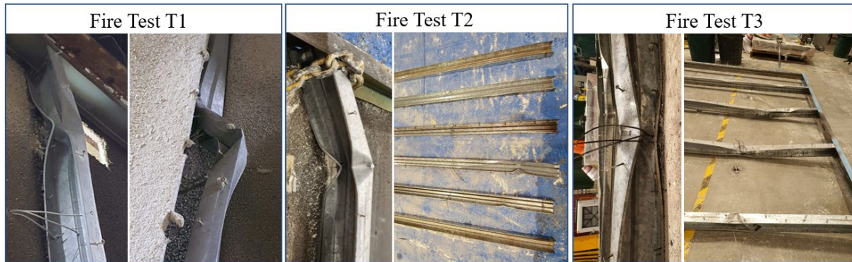
Fig. 8. Distortional buckling failures of tested LSF walls.
