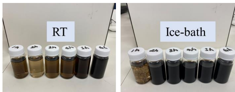
Figure 4. 5 Sample vials containing GO -1 hr, GO-2hr, GO-3hr, GO-4hr, GO-5hr and GO-6hr subject to ultrasonication at room temperature (Image on the left) and at ice bath (0-4°) (Image on the right)
