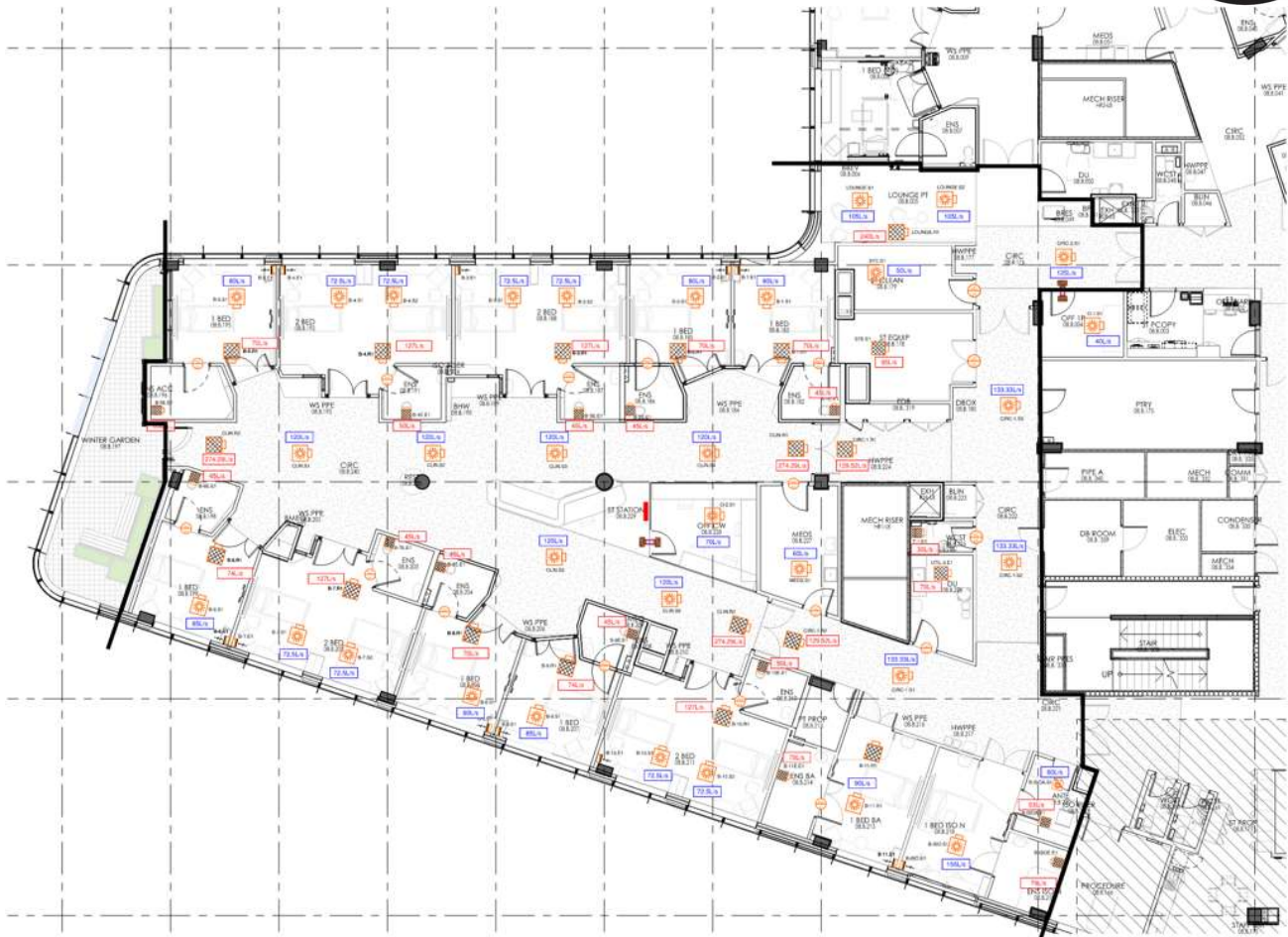
Figure 4-7 Mechanical system for scenario 3 (localised return)
