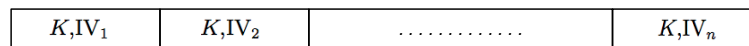
Figure 2.4: A keystream generated using the same secret key, K , and multiple IVs
